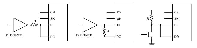
Figure 3. Possible Configurations to Minimize Problems Due to READ Contention
