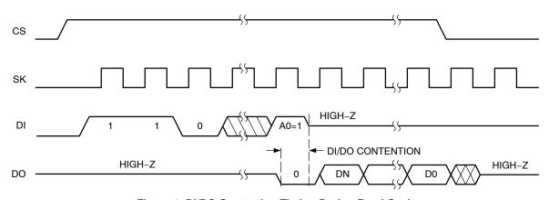
Figure 1. DI/DO Contention Timing During Read Cycle
