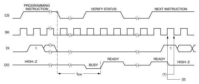
Figure 4. Programming Instruction and Status Reset with 4-Signal Interface
